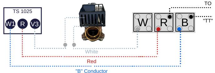
AUTOMAG RS260 TWO-WIRE OPTION (RETIRED THERMOSTAT)
